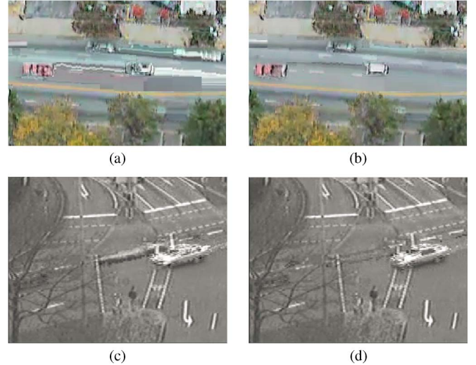
Fig. 5. Sample concealed frame for (a) and (b) “Camera6” sequence and (c) and (d) “dt_passat” sequence. (a) BMA-concealed frame. (b) MC-concealed frame. (c) BMA-concealed frame. (d) MC-concealed frame.
