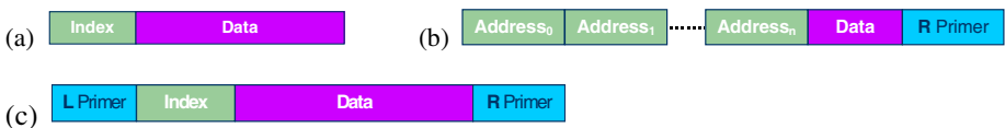
Fig. 1. Commonly used database elements (DE): (a) An index-data DE; (b) An address based DNA DE approach; (c) A DNA DE with left and right primers added for easy replication. All single border rectangles represent single stranded sequences.
